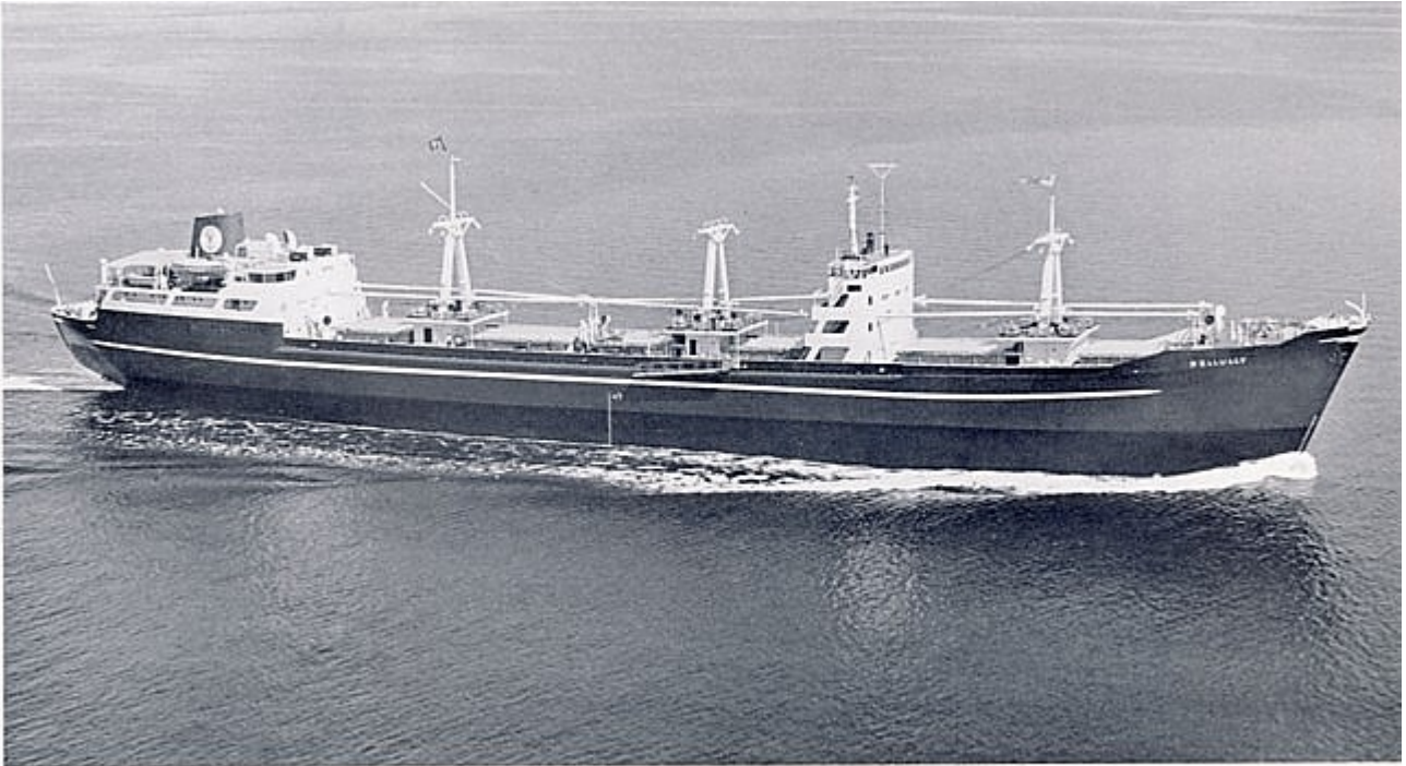
M.S. BELLULLY, cargo motorship 13,400 tons d.w., 14½ knots.
